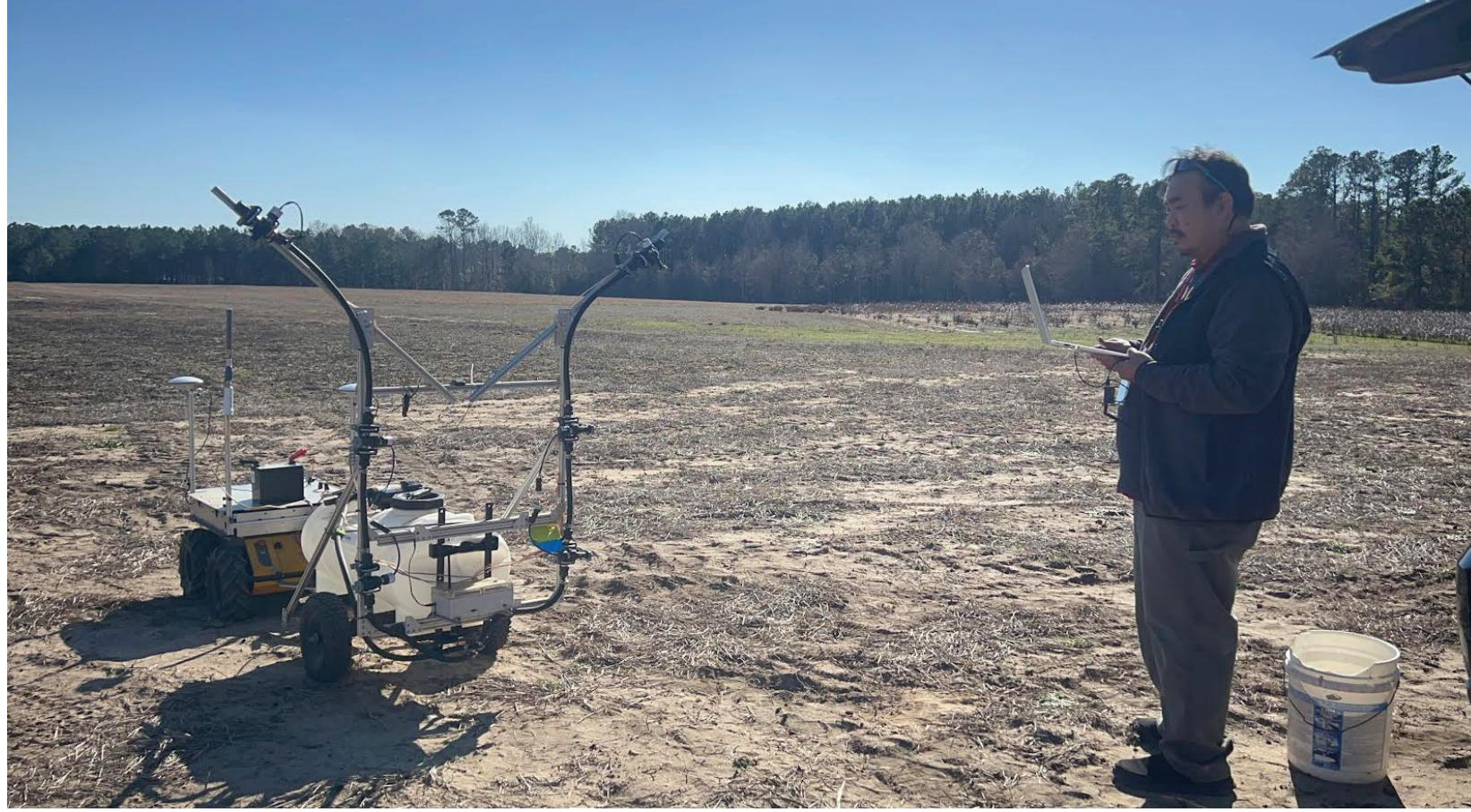
**TECH.** Van Patiluna demonstrates the autonomous defoliator, controlling the precision sprayer through a program on his laptop, which allows farmers to customize applications for greater efficiency and reduced chemical use. (Photo C/O Melissa Foust-McCoy)
