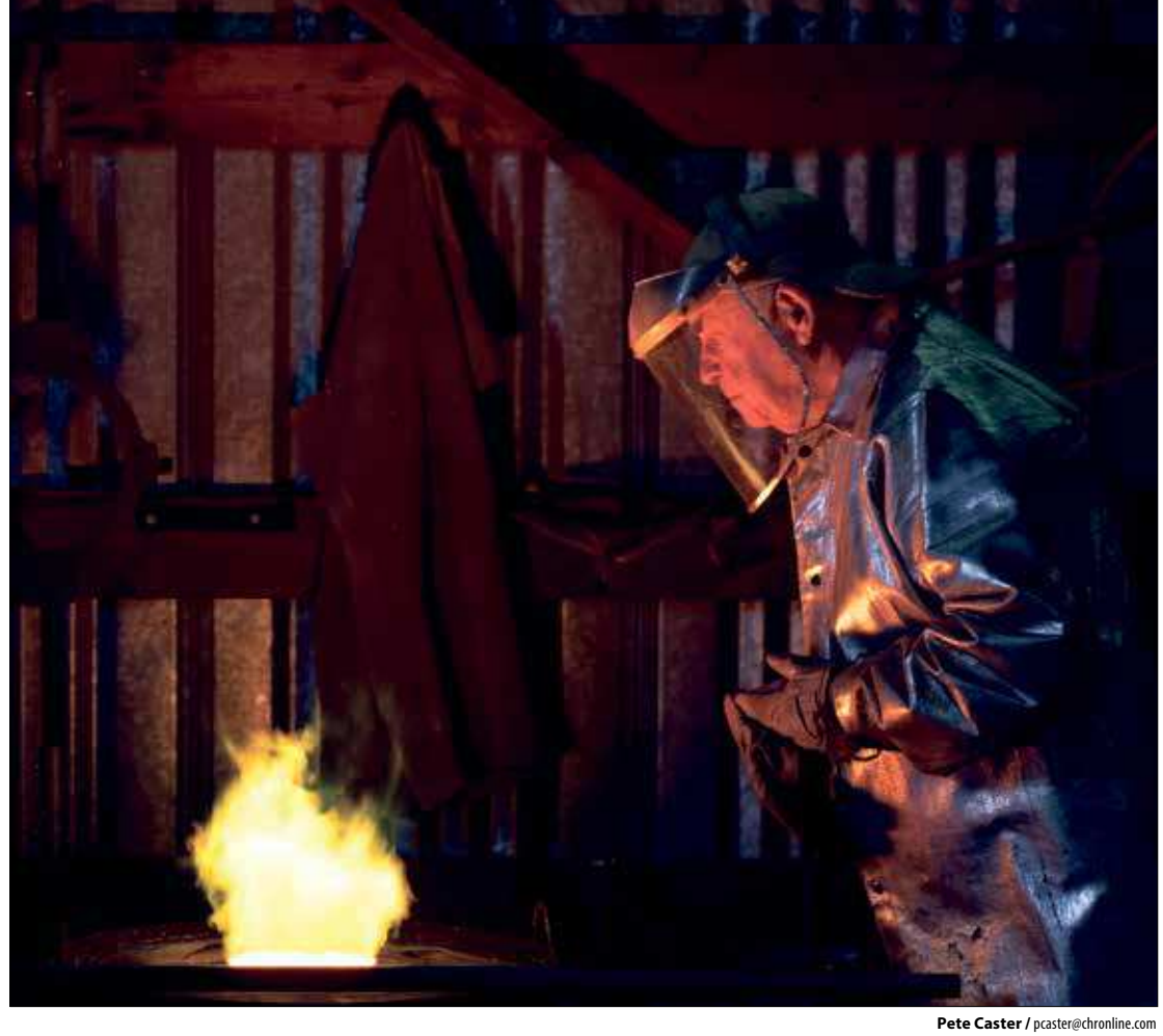
Jim Stafford, a local bronze sculptor, looks into the furnace where a crucible containing liquid bronze is heated to 2,150 degrees prior to pouring the metal into molds on Saturday afternoon at his shop in Adna.
