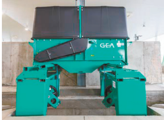
Elevated SW Cable Drive Unit
